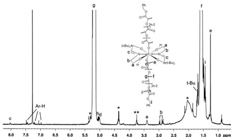
**Fig. 6**  $^1\text{H}$  NMR spectrum of poly(D,L-lactide) with terminal benzyl ester group and  $[(\text{dME})_2(\text{HIM})\text{P}]_2\text{Ti}(\text{IV})$  complex [\*a few poly(D,L-lactide)s with terminal benzyl ester group; \*\*methylene proton peaks of rudimental ethanol;  $[\text{M}]_0/[\text{Ti}]_0/[\text{BnOH}]_0 = 400:1:2$ , at  $160^\circ\text{C}$  for 12 h]
