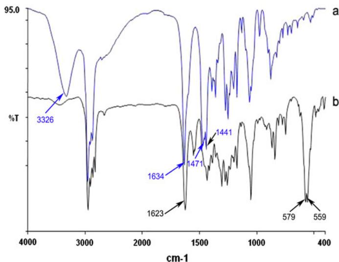
**Fig. 2** The comparison of FTIR spectra for (dME)<sub>2</sub>(HIM)P-H<sub>2</sub> ligand (*a*) and [(dME)<sub>2</sub>(HIM)P]<sub>2</sub>Ti(IV) complex (*b*)
