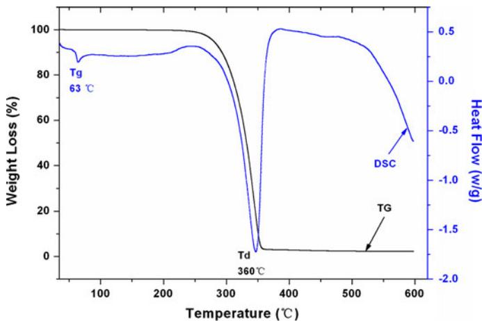
**Fig. 8** TG and DSC analysis of the poly(D,L-lactide) with  $[(\text{dME})_2(\text{HIM})\text{P}]_2\text{Ti}(\text{IV})/\text{BnOH}$  as a binary catalyst
