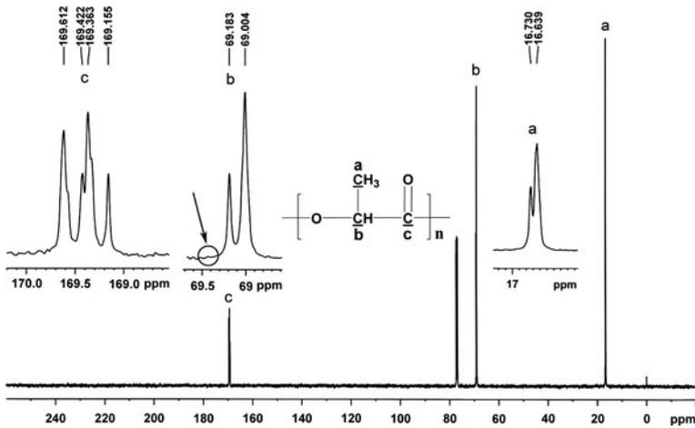
**Fig. 7**  $^{13}\text{C}$  NMR spectrum of obtained poly(D,L-lactide) with  $[(\text{dME})_2(\text{HIM})\text{P}]_2\text{Ti}(\text{IV})/\text{BnOH}$  as a binary catalyst (no visible peak of *iss* stereosequence at 69.4 ppm)
