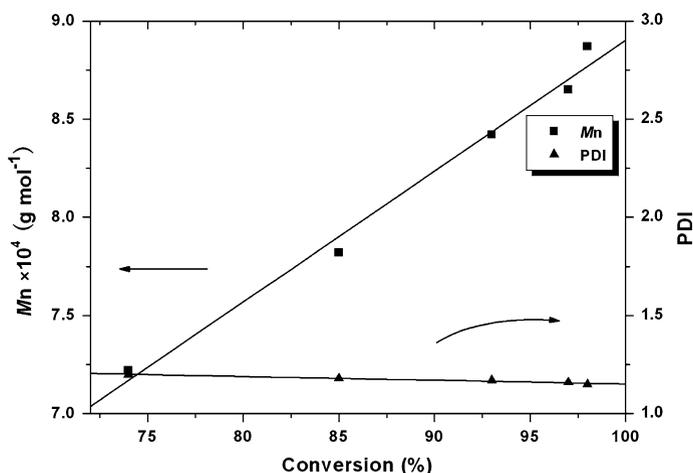
**Fig. 5** Plot of  $M_n$  (■) and PDI (▲) versus monomer conversion for ROP of D,L-lactide catalyzed by a binary catalyst [(dME)<sub>2</sub>(HIM)P<sub>2</sub>Ti(IV)/BnOH (bulk phase, 160 °C,  $[M]_0/[Ti]_0/[BnOH]_0 = 1,600$ , here M: D,L-lactide monomer, Ti: [(dME)<sub>2</sub>(HIM)P<sub>2</sub>Ti(IV) complex, BnOH: benzyl alcohol)
