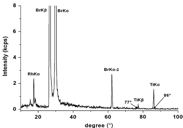
**Fig. 1** XRF spectroscopy of  $[(dME)_2(HIM)P]_2Ti(IV)$  complex
